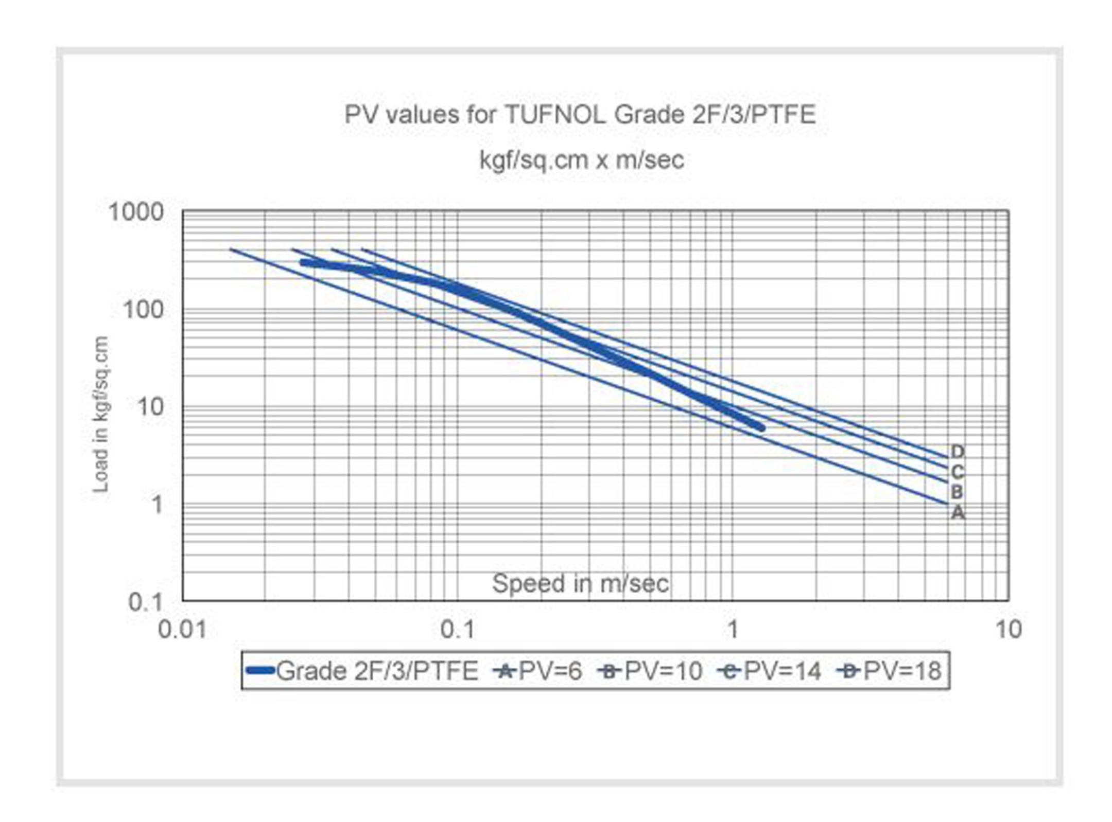
The PV values shown in Figure 1 represent the highest values which unlubricated specimens of TUFNOL Grade 2F/3/PTFE withstand in laboratory testing. The test specimen is a rectangular block with one face machined to provide a cylindrical bearing surface which is run against a 35 mm diameter hardened steel ring.
